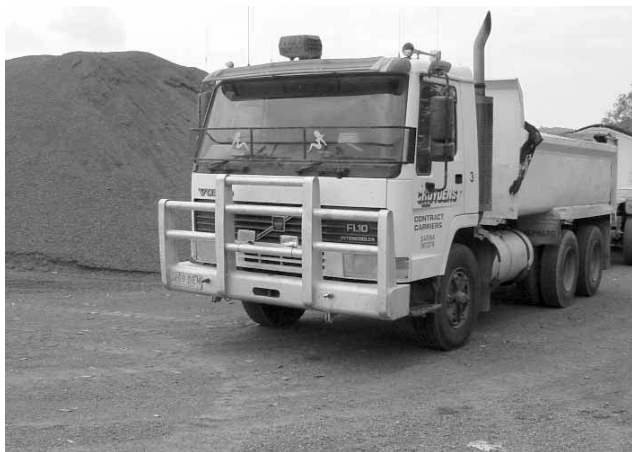
A Volvo FM10 heavy duty truck operated by Croydens, a CSR sub-contractor, which is running on diesohol E15 as a trial begun last year.
